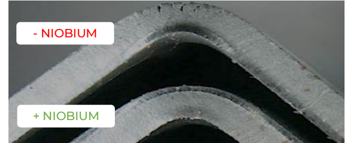
IMPROVED FLAT SHEET FORMABILITY WITH NIOBIUM 4
