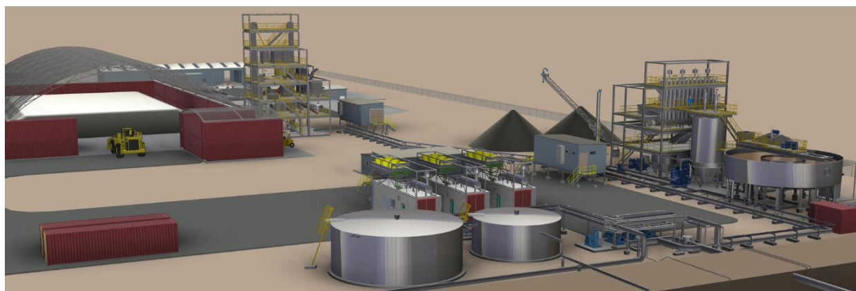
Figure 3 Fungoni Preliminary 3-D Engineering Design, based on modular relocatable design concept
