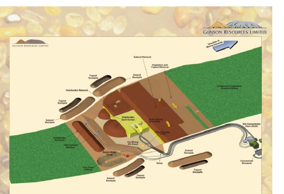
COBURN MINERAL SAND PROJECT MINING METHOD SCHEMATIC - SEQUENCE 5
