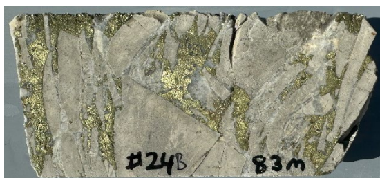
High grade chalcopyrite infill in hornfels breccia. CAE Hole 24, 83m . 2m interval 82m-84m : 3.04% Cu, 0.23 g/t Au, 102.9 g/t Ag, 4.11% S (2m @ 4.0% CuEq).
