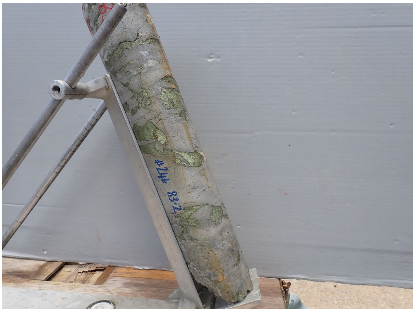
Fig 12. Photo full HQ core Hole #24, oriented in core oriented frame at 83.2m, hole drilling to west south west , view looking south east , hole at 83m inclined at -68 degrees toward 248 degrees mag: Chalcopyrite rich Hydrothermal Infill Breccia. Clasts dominated by yellow grey, sericite altered hornfels, with infill of chalcopyrite (golden) , pyrite (brassy) ,minor calcite (white) ,quartz (glassy).
