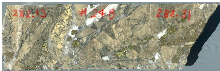
High grade chalcopyrite infill in hornfels breccia. CAE Hole 24, 83m . 2m interval 82m-84m : 3.04% Cu, 0.23 g/t Au, 102.9 g/t Ag, 4.11% S (2m @ 4.0% CuEq).
