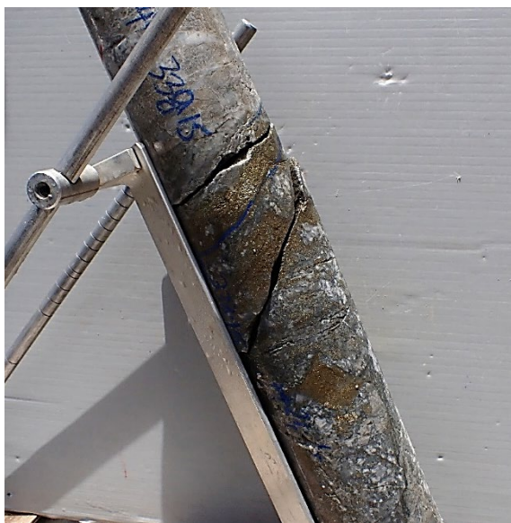
Fig 13. Photo full HQ core Hole #24 ,157.2m, oriented in core oriented frame, hole drilling to west south west , view looking south east , hole at 157m inclined at -68 degrees toward 251 degrees mag: Infill hydrothermal breccia, with slabby/shingle clasts aligned normal to direction of hole. Slab alignment averages dipping 45 degrees, striking 010 degrees mag , dip direction 100 degrees mag. Clasts dominated by light grey,sericite altered hornfels , with infill of carbonate (white) , quartz (colourless), chlorite infill & altered rock flour (green) , pyrite (brassy) . 1m Interval 157m-158m grades 0.53%Cu, 0.13 g/t Au, 8 g/t Ag, 3.09% S.
