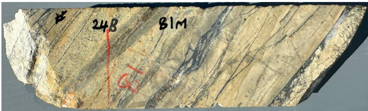
Fig 11. Photo Half HQ Core . Hole 25CAEDD024 at 81m - sericite altered and heavily veined hornfelsed siltstone with prominent sheeted veins of quartz-ankerite-pyrite-molybdenite -minor chalcopyrite. -1m interval 81m-82m : 666 ppm Mo, 0.11% Cu, 0.02 g/t Au, 1.3 g/t Ag, 0.5% S.
