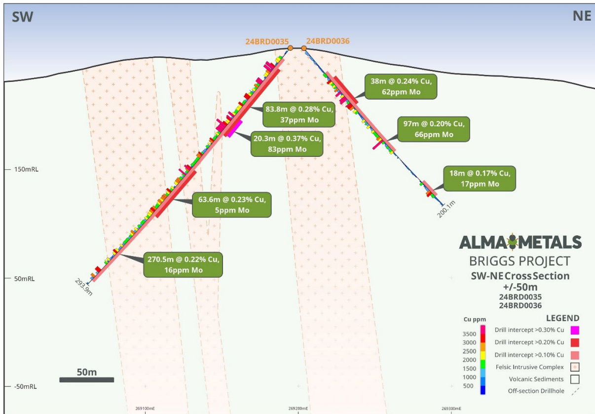
Figure 6. Cross-Section showing hole 24BRD0035 and 24BRD0036, testing the Southern Porphyry Target. For location of cross-section, refer to Figure 1.
