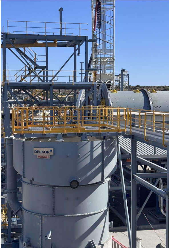
Photos 3 and 4. New ball mill successfully installed at Eloise copper mine, with the new rougher flotation cell in the foreground (left); and subsequent installation of the primary cyclone cluster (right).
