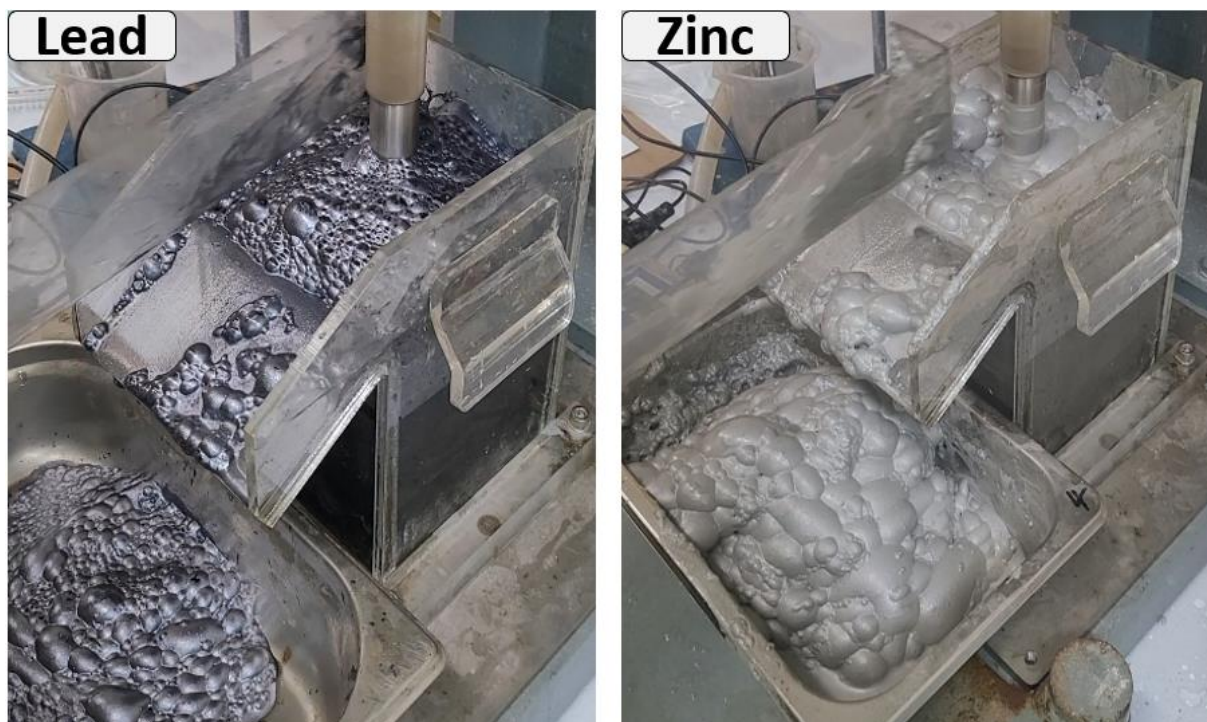
Figure 4 – Lead Rougher (LHS) and Zinc Cleaner (RHS) tests showing flotation of zinc and lead sulphides.
