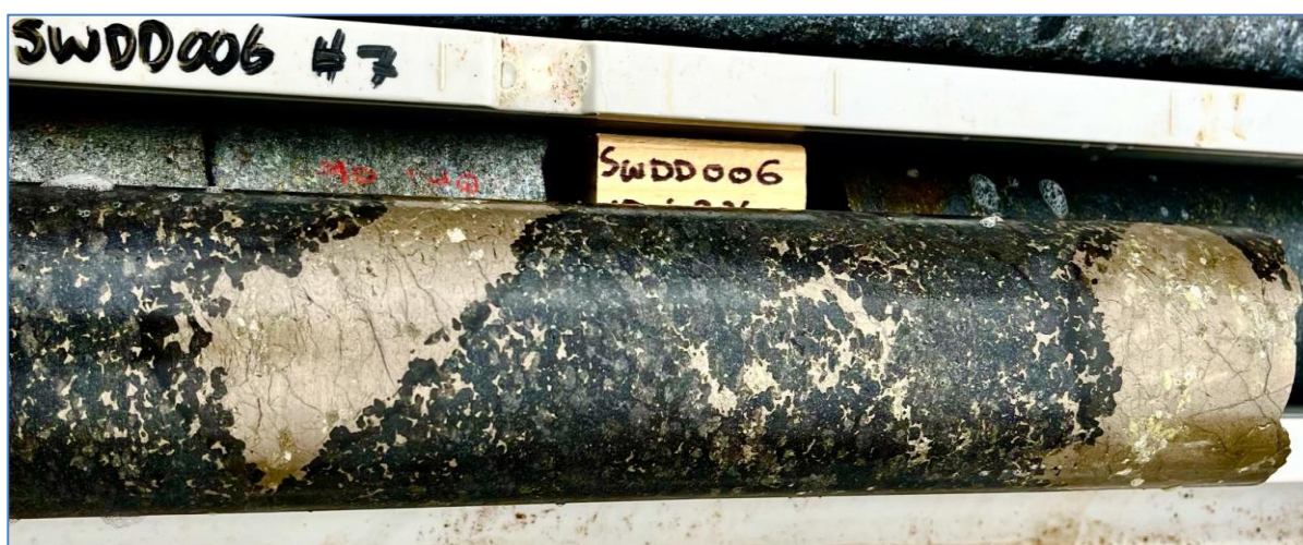
Figure 1. Drill core from hole SWDD006 (226.55 – 226.85 m) showing net-textured to semi-massive magmatic sulfide mineralisation composed predominantly of pyrrhotite, pentlandite, and chalcopyrite.
