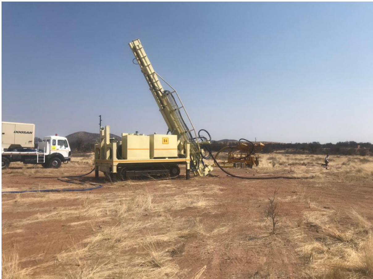
Figure 2: FerroDrill on site drilling at Otjiwaru, targeting sub-cropping malachite mineralisation.
