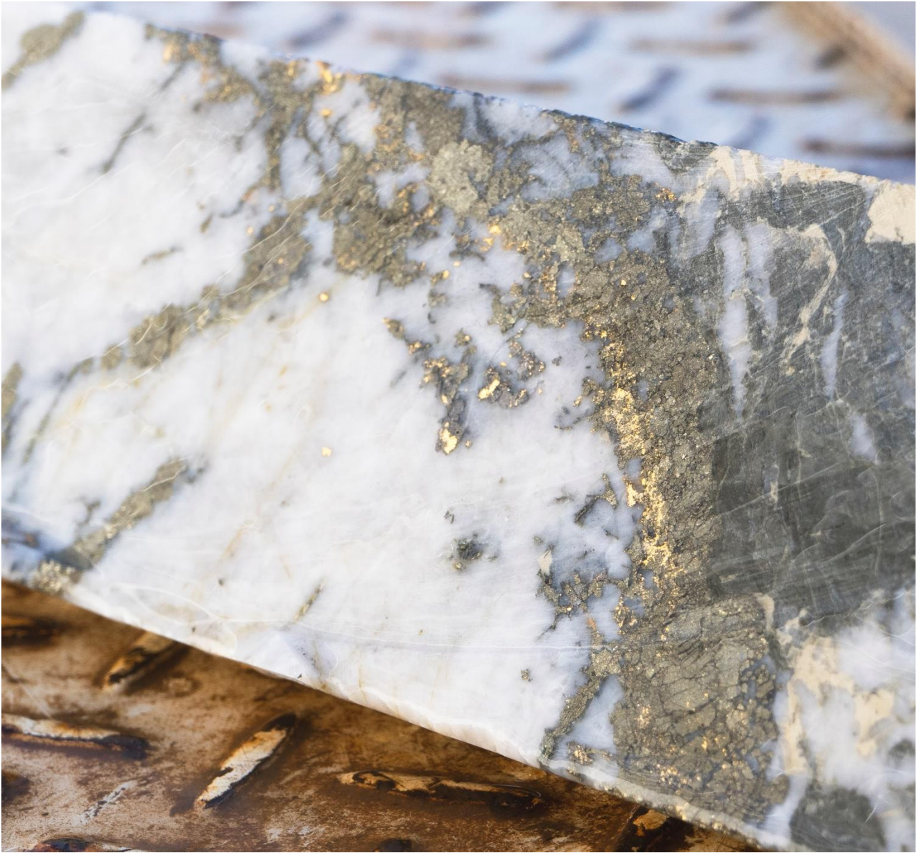
Figure 3. Close-up photo of previously drilled core from hole HVD003 (~190.5m down hole) at Happy Valley. The ultra-high grade mineralisation in the photo includes abundant visible gold (yellow) hosted with sulphides (brass-colour) and quartz (white) and graded 0.6 metres at 2,430g/t Au . Full details of the previous drilling can be found in the Advance Metals' ASX release dated 6 January 2025. Ends.
