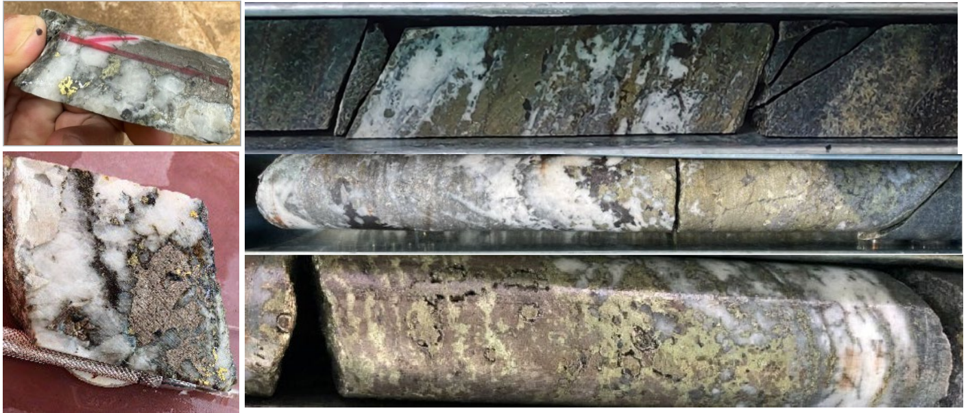
Figure 14 | Mineralised veins in Memot diamond core. Quartz veining with Pyrite, Arsenopyrite, Pyrrhotite, Chalcopyrite and Sphalerite sulphides. In order from Left hand photos: DD24MMT243 - 1m @ 2,090.00g/t Au from 130m. Right Hand Side Top to Bottom DD21MMT001 - 1m @ 8.91g/t Au, 2.16% Cu from 48m, DD22MMT013 - 0.4m @ 17.70g/t Au, 230g/t Ag, 2.78% Cu, 0.56% Pb and 1.74% Zn from 190m and DD21MMT006 - 1m @ 25.4g/t Au, 73g/t Ag, 1.81% Cu, 0.1% Zn
