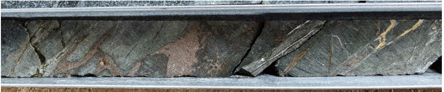
Figure 8 | Mineralised veins in Okvau diamond core. Hydrothermal breccia with pyrrhotite sulphides within a hornfels sedimentary package - 6m @ 7.34g/t Au from 234m (RCDD25OKV776). The section of core in the image was part of a 1 metre intercept grading at 33.40g/t Au
