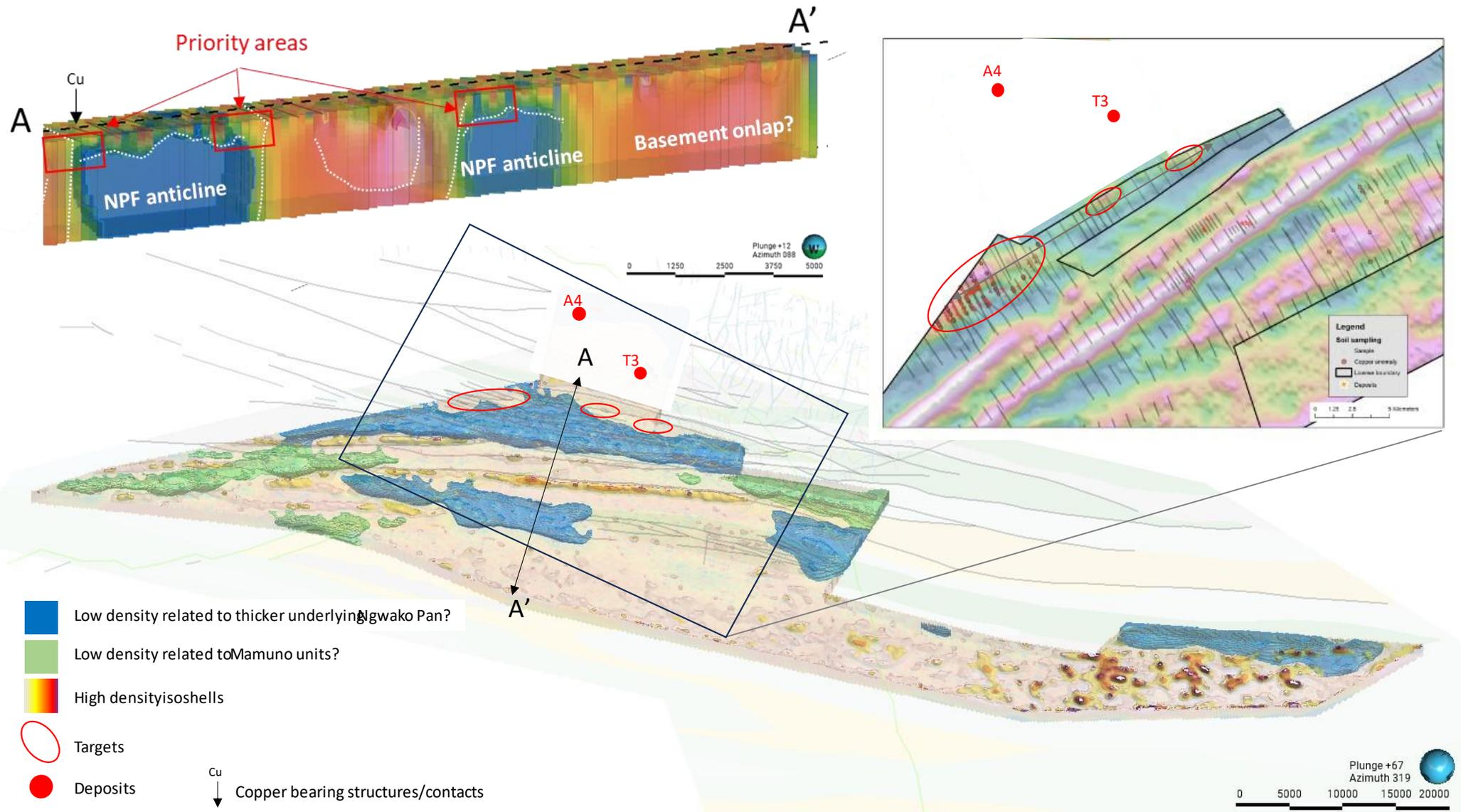
**Figure 3. 3D oblique view of AGG tensor density inversion results over KITE (and a portion of Sandfire's Motheo Production Hub). Selected sections through the density inversion model and inset of residual filtered gravity have been included to highlight underlying potential anticlinal features and structurally controlled dense targets. Note the spatial proximity to Sandfire's T3 and A4 deposits.**
