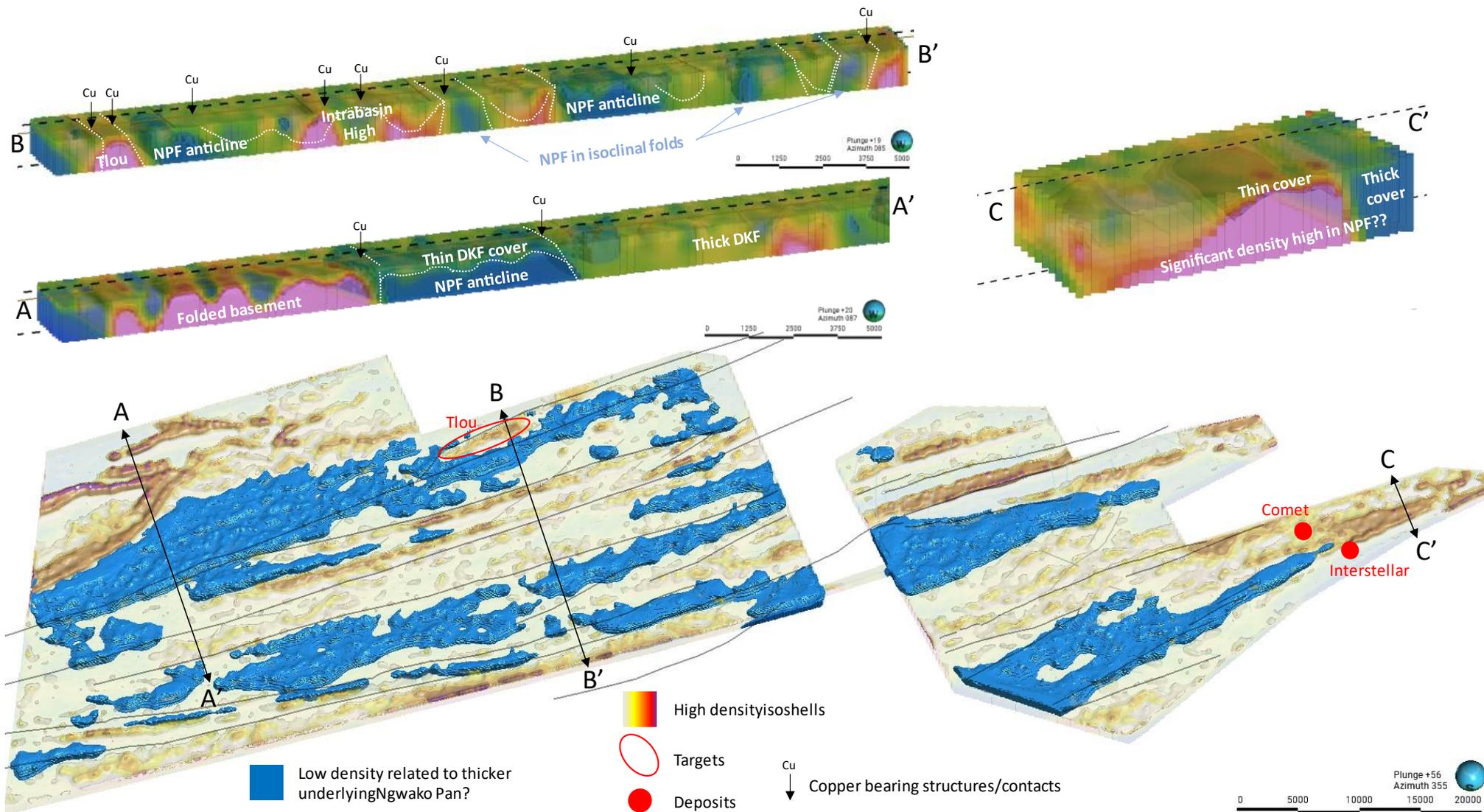
**Figure 1. 3D oblique view of AGG tensor density inversion results over KITW and NCP. Selected sections through the density volume highlight key results from the data. The evidence for copper bearing structures on the margin of potential anticlinal structures with the redox contact preserved in the fold hinge is compelling. Clear dense bodies associated with the Tlou Target and footwall in proximity to Comet and Interstellar targets may provide an additional targeting layer.**
