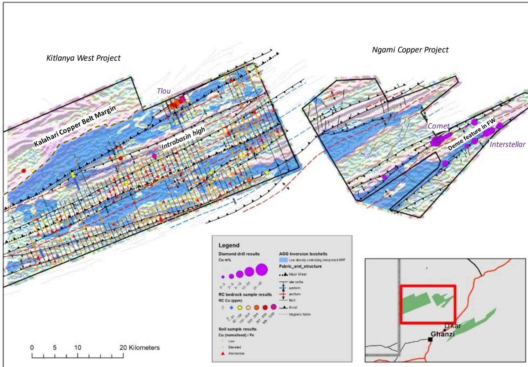
**Figure 2.** Low density zones overlain on a rotational invariant image product from the AGG tensor results. Anomalous soil sample, bedrock drilling and diamond drill results overlain. Note the excellent correlation with anomalous results and the structurally controlled margins of the low-density zones. Results provide a substantial step forward in target prioritisation.
