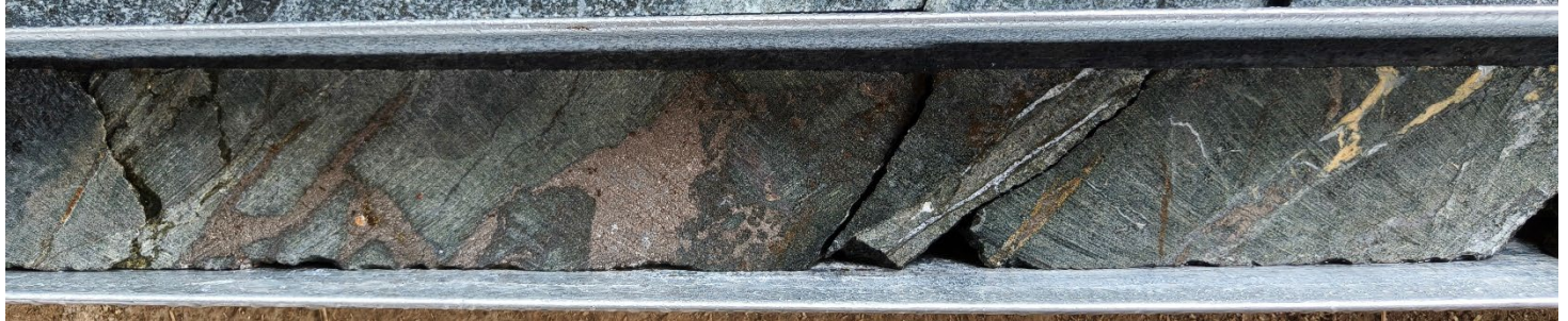
Figure 12 | Mineralised veins in Okvau diamond core. Hydrothermal breccia with pyrrhotite sulphides within a hornfels sedimentary package - 6m @ 7.34g/t Au from 234m (RCDD25OKV776). The section of core in the image was part of a 1 metre intercept grading at 33.40g/t Au
