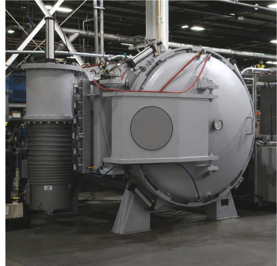
Sintering furnace (example of model, currently in fabrication)
