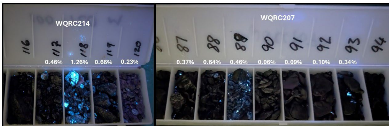
Figure 3 – WQRC214 (left) and WQRC207 (right) chip trays under UV light demonstrating the relationship between scheelite mineralisation in chips and their associated tungsten (WO 3 %) laboratory assays
