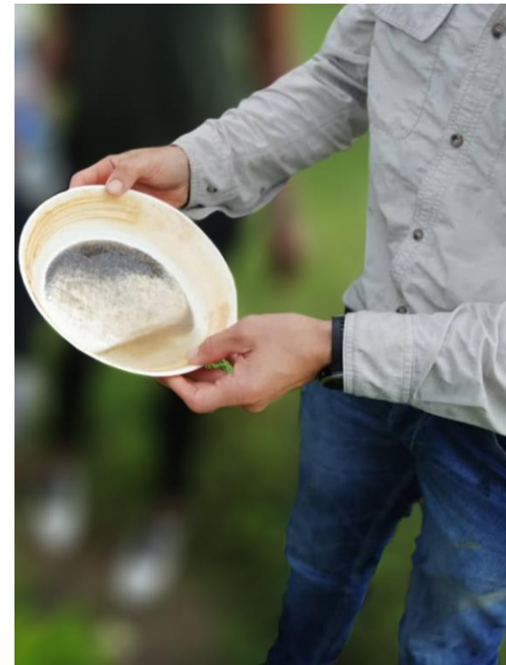
Image: Fungoni surface pan sample showing extremely high grade HM
