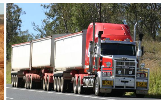
Image: Typical Triple Road Train Configuration
