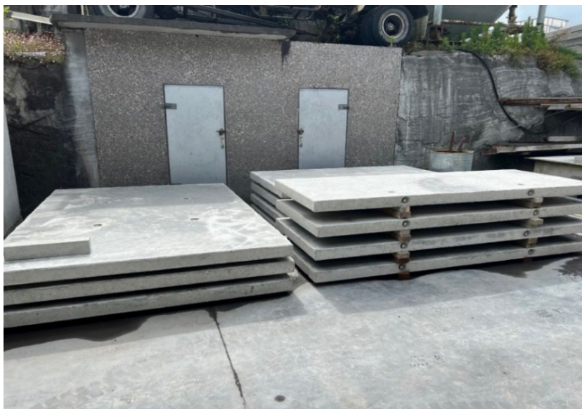
Figure 3: Graphene-enhanced cement slabs to be used as insulation panels and tested in a commercial project.
