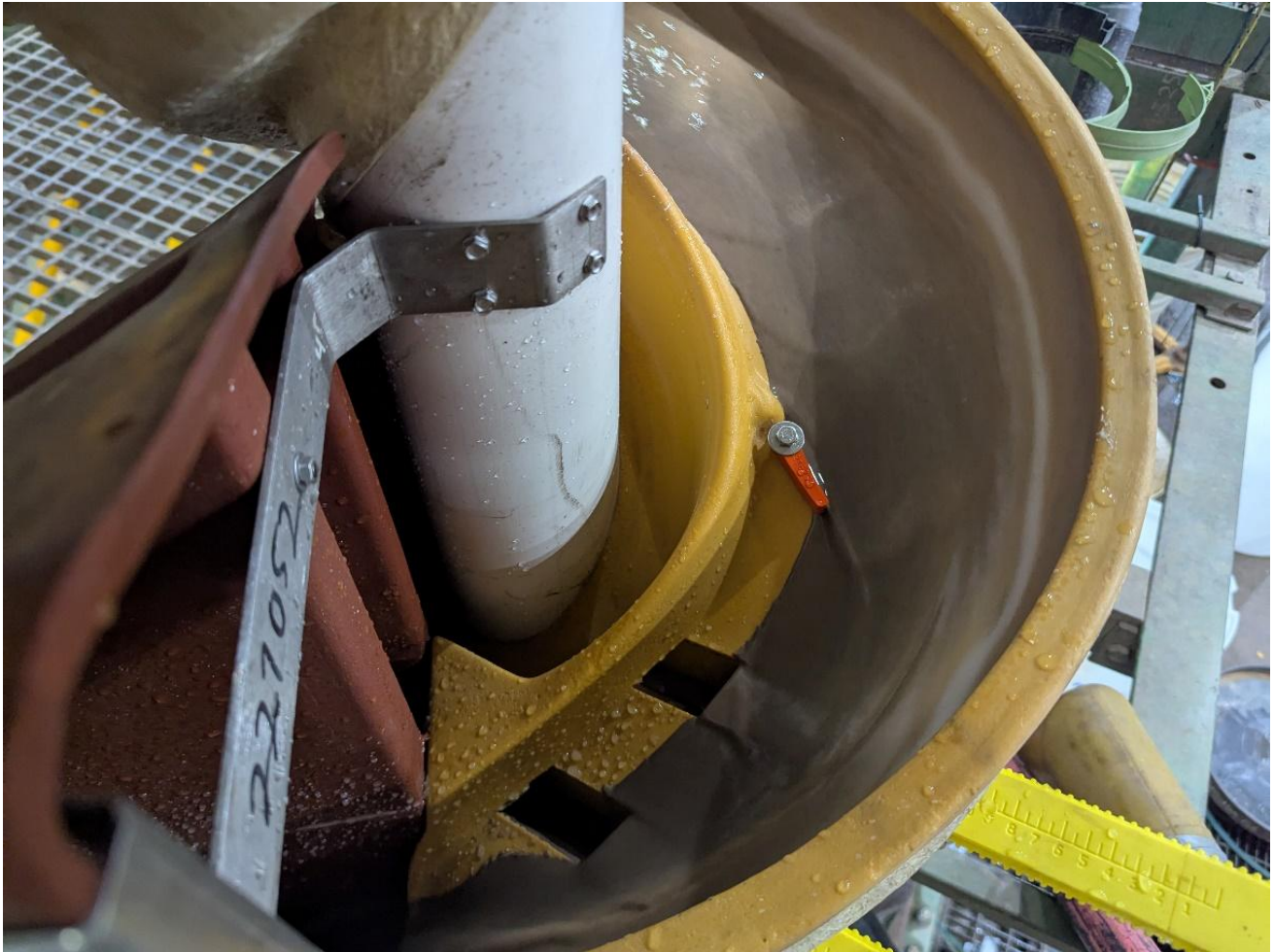
Figure 2: HG10i spiral processing concentrate from the rougher spirals
