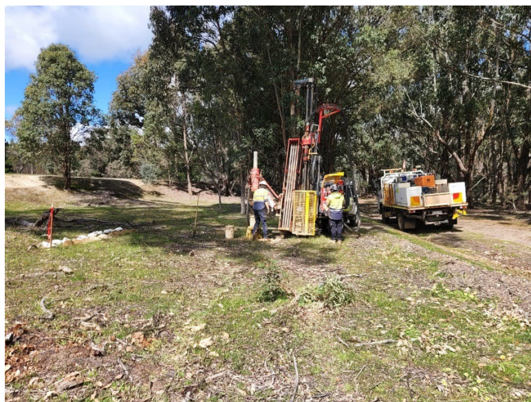
Figure 2. Aircore drilling underway at the Ivar Prospect, WA
