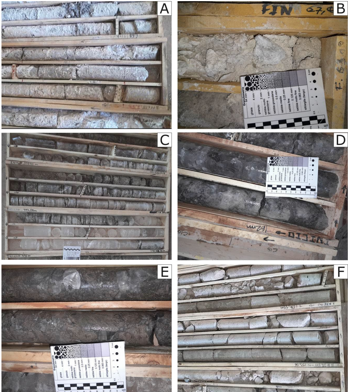
Figure 5 – Main lithologies as described in hole DDH-1. A: Sulphates B: Sand with gypsum. C: Discoidal Halite. D: Halite with matrix. E: Sand with gypsum. F: Sand
