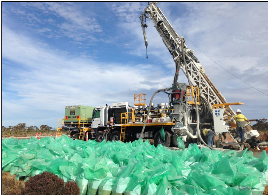
Figure 9: RC drill rig over C1
