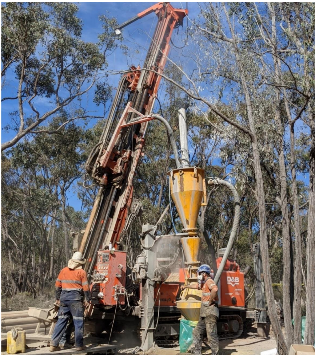
Figure 7: RC drilling at Fentiman's Reef prospect, South Muckleford Gold Project
