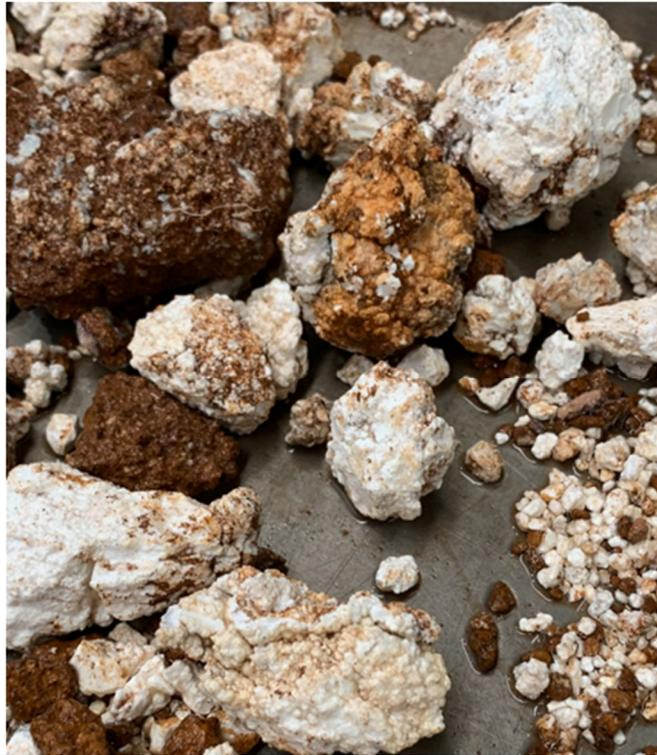
**Figure 3. Coarse Material containing calcite, magnesite and gibbsite.**
