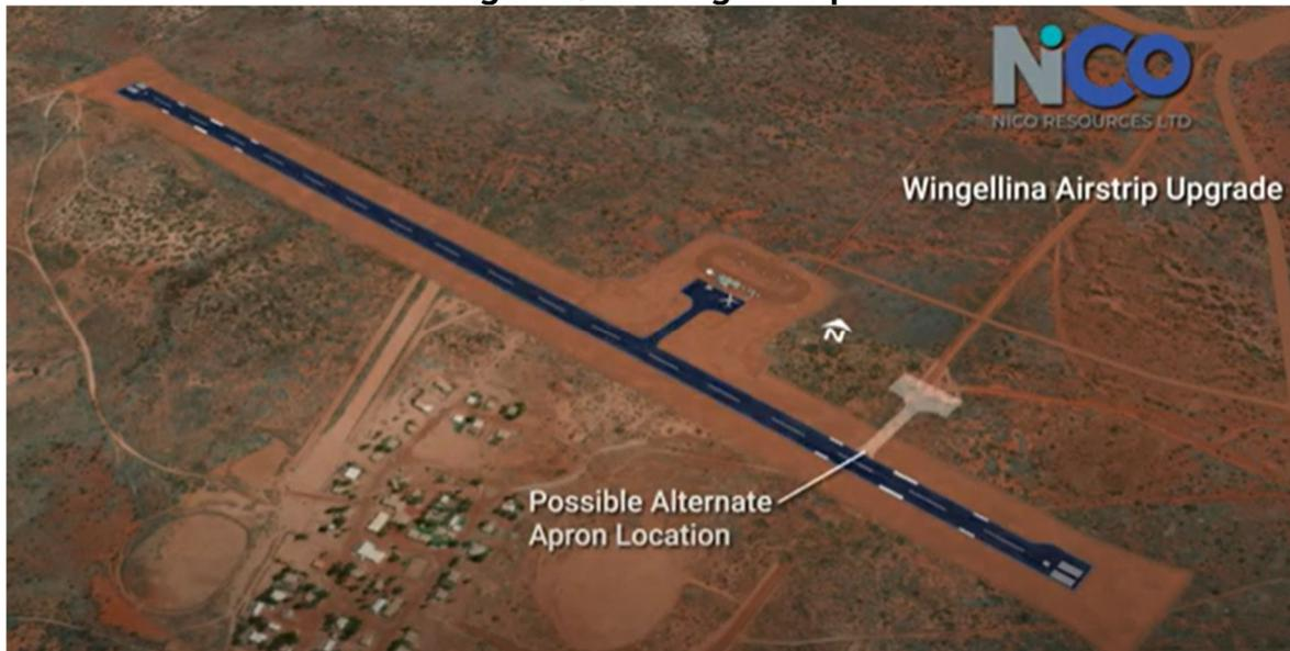
**Figure 11. New proposed code 4C airstrip**
