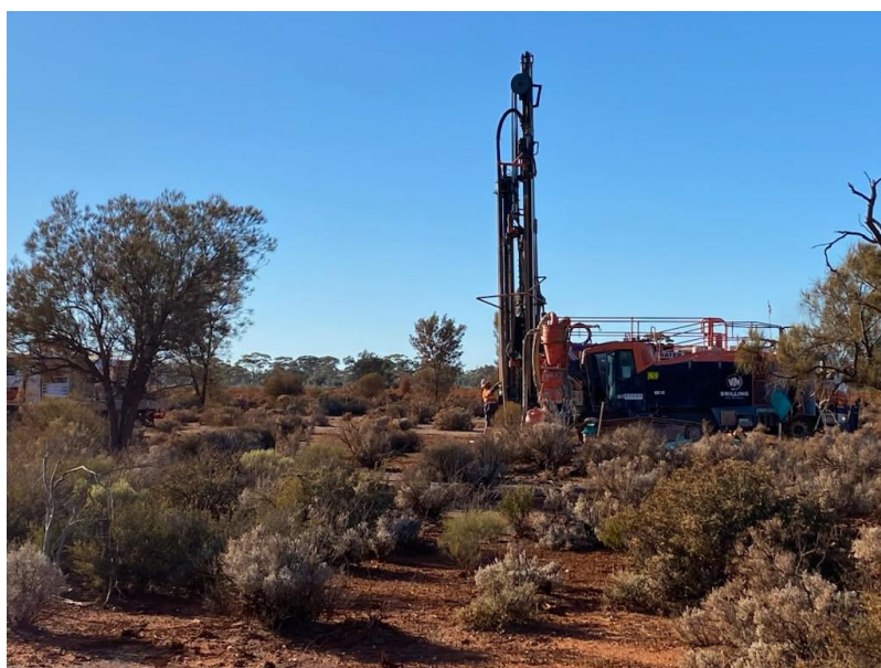
Figure 2: Figure showing the VM Drilling Epiroc ROC L8 track mounted RC rig at the Majestic North gold project.
