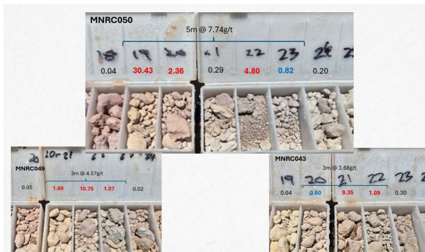
Figure 1: Photographs of the RC chips for holes MNRC043, MNRC049 and MNRC050 showing the assay results for the 1m interval against the logged geology.
