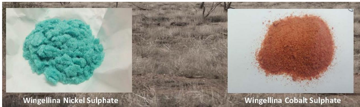
Figure 7: Battery Grade Sulphates precipitated from Wingellina ore in 2017
