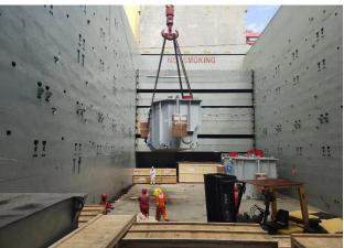
Figure 7: Transformers Loaded into Ship Enroute to Site
