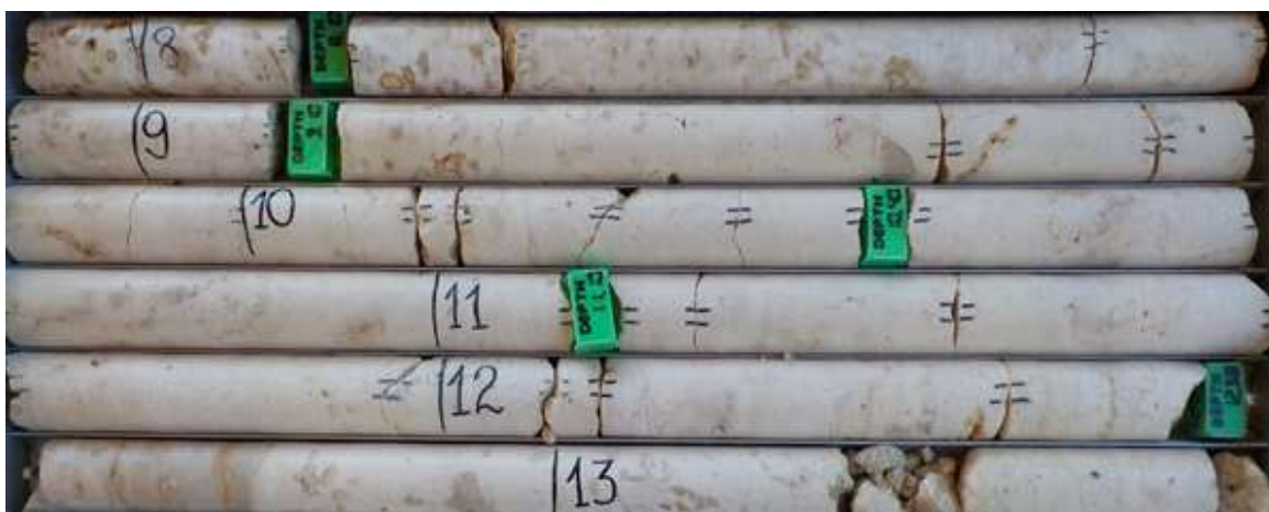
Fig 1 - Soalara Limestone Core - High purity @ 97% Calcium Carbonate
