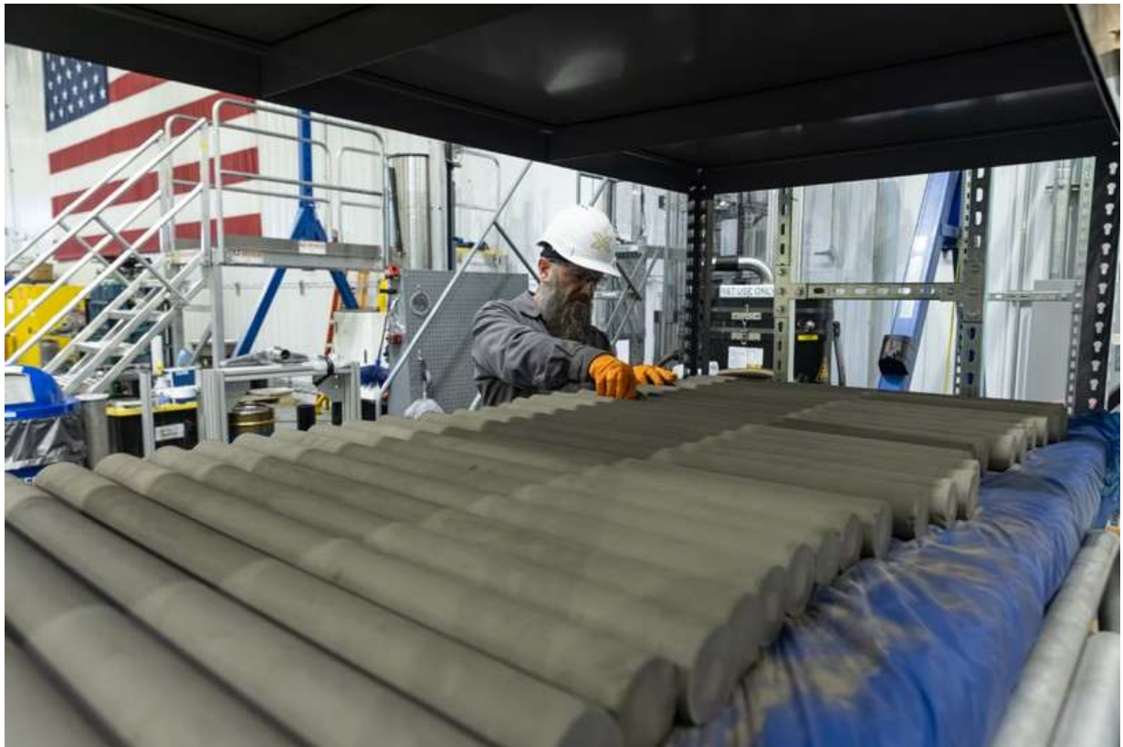
Figure 7: Production of “green parts” from IperionX titanium metal powder prior to HSPT™ sintering
