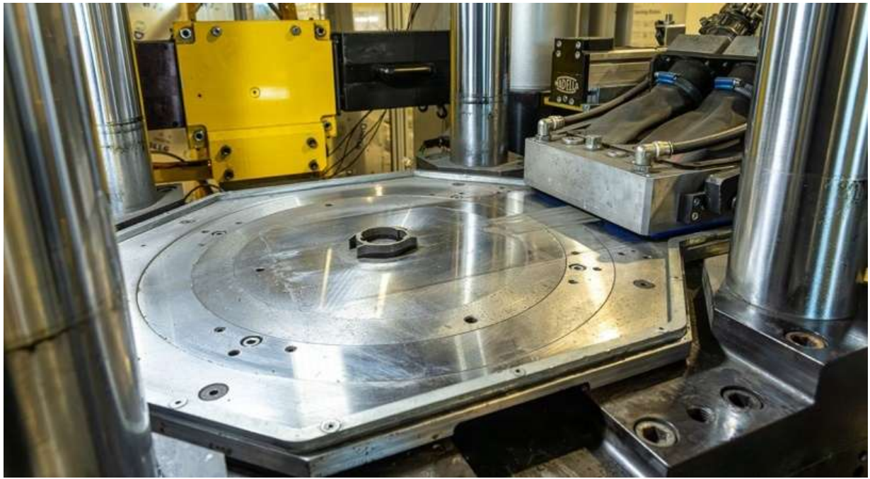
Figure 5: Six-axis 300-ton SACMI press in operation
