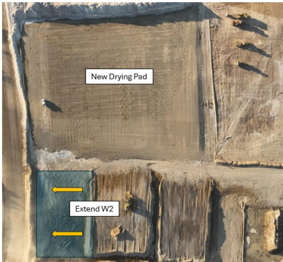
**Image 2:** Northern drying pads. Used for <12% moisture for final solar drying.
