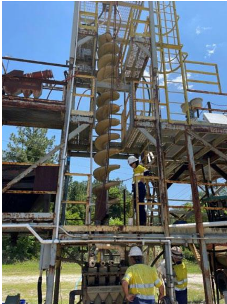
Figure 1: Spiral Test Work at Minerals Technologies
