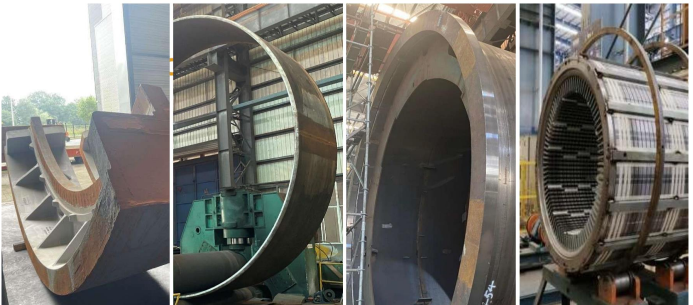
Figure 6: Fabrication of ball mill and ring gear segments
