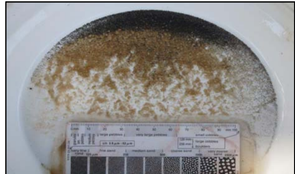
Figure 3. Pan sample of the 0.5m thick high grade cross bedded strand at Madimba East with an estimated THM content of > 5% THM. Mineral sands are identified as the black mineral at the top of the pan. All samples are panned for estimation of THM% from a standard sized sample to ensure visual calibration is maintained.
