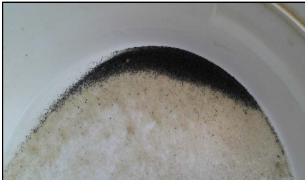
Figure 2. Pan concentrate sample from Madimba East – MTPA068 with a visual pan estimate >4% THM. Heavy mineral is located on the top of the pan as the dark coloured or black grains. All samples are panned for estimation of THM% from a standard sized sample to ensure visual calibration is maintained.
