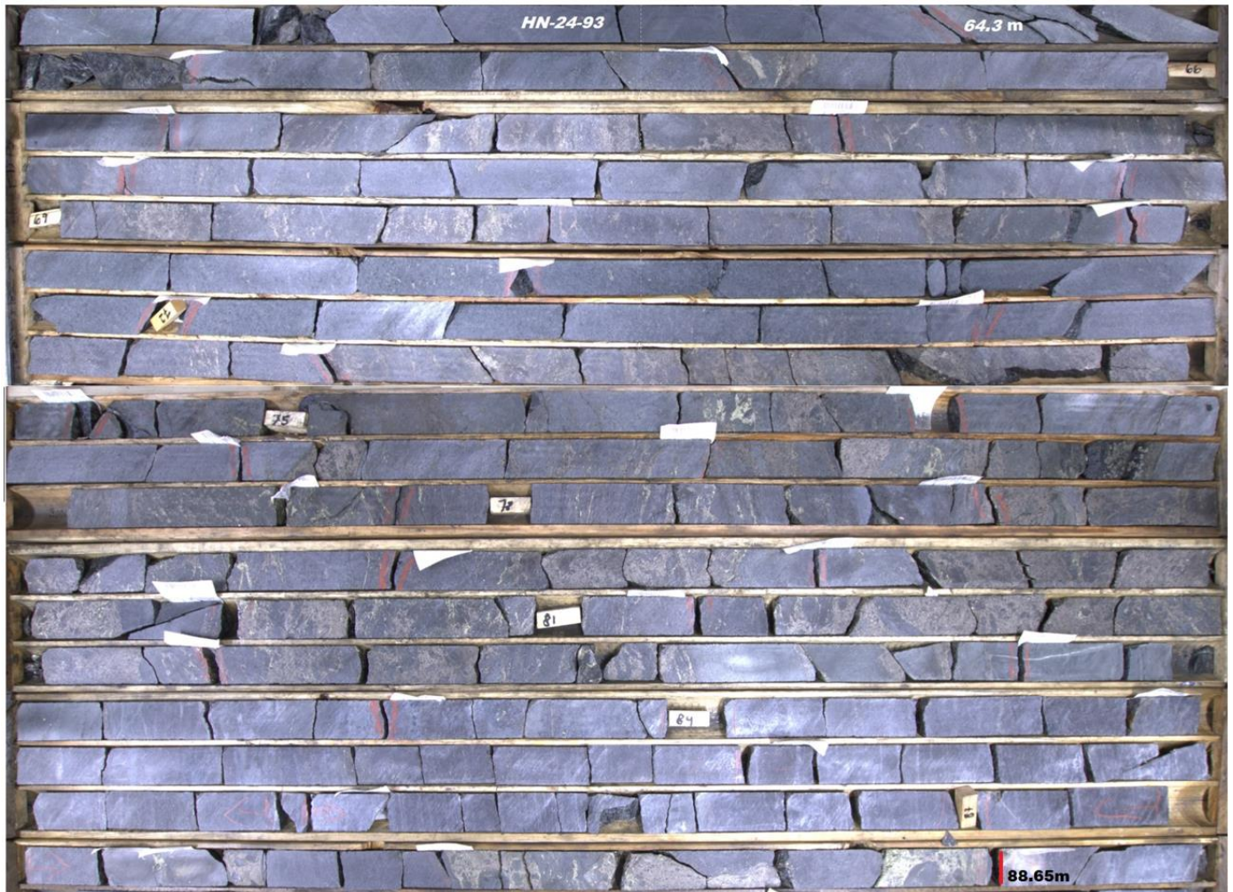
Figure 4: HN-24-93 Core Photo 64.3-88.65 showing pyrrhotite, chalcopyrite, pyrite, pentlandite semi-massive to massive sulphides in melano-gabbro, mafic dyke and meta-sediments
