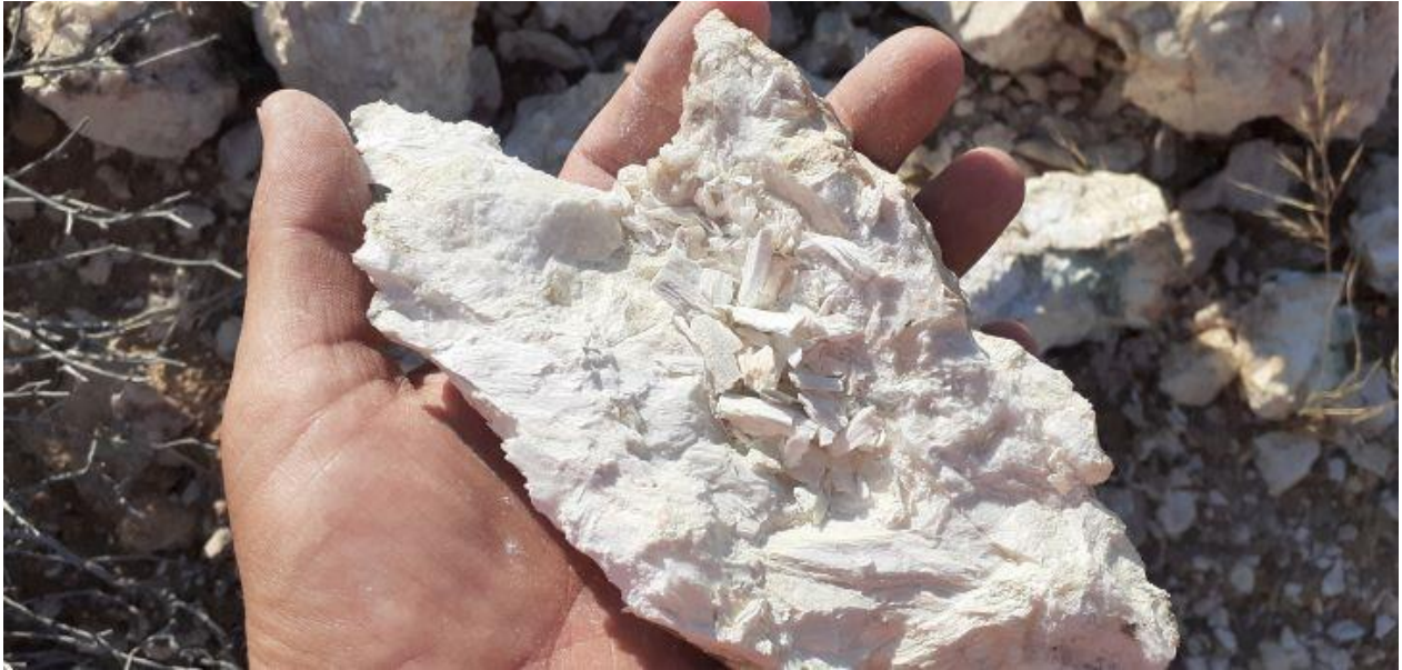
Figure 1: Example of unaltered spodumene identified at surface at the large tin mine working on EPL 8535 [Uis Lithium Project] - Note: Visual estimates should not be considered a proxy or substitute for laboratory analysis. Assay results are expected to be received in January 2023, subject to turnaround times at the laboratory. Sample Tag: U4681; Sample location – E: 472219 and N: 7639525
