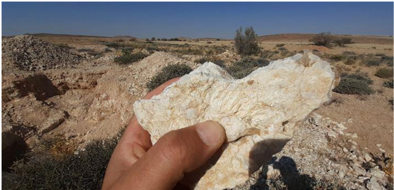
Figure 2: Large pegmatite mine working with an example of unaltered spodumene identified at surface at the mine workings on EPL 8535 [Uis Lithium Project] - Note: Visual estimates should not be considered a proxy or substitute for laboratory analysis. Assay results are expected to be received in January 2023, subject to turnaround times at the laboratory. Sample Tag: U4672; Sample location – E: 472460 and N: 7639905
