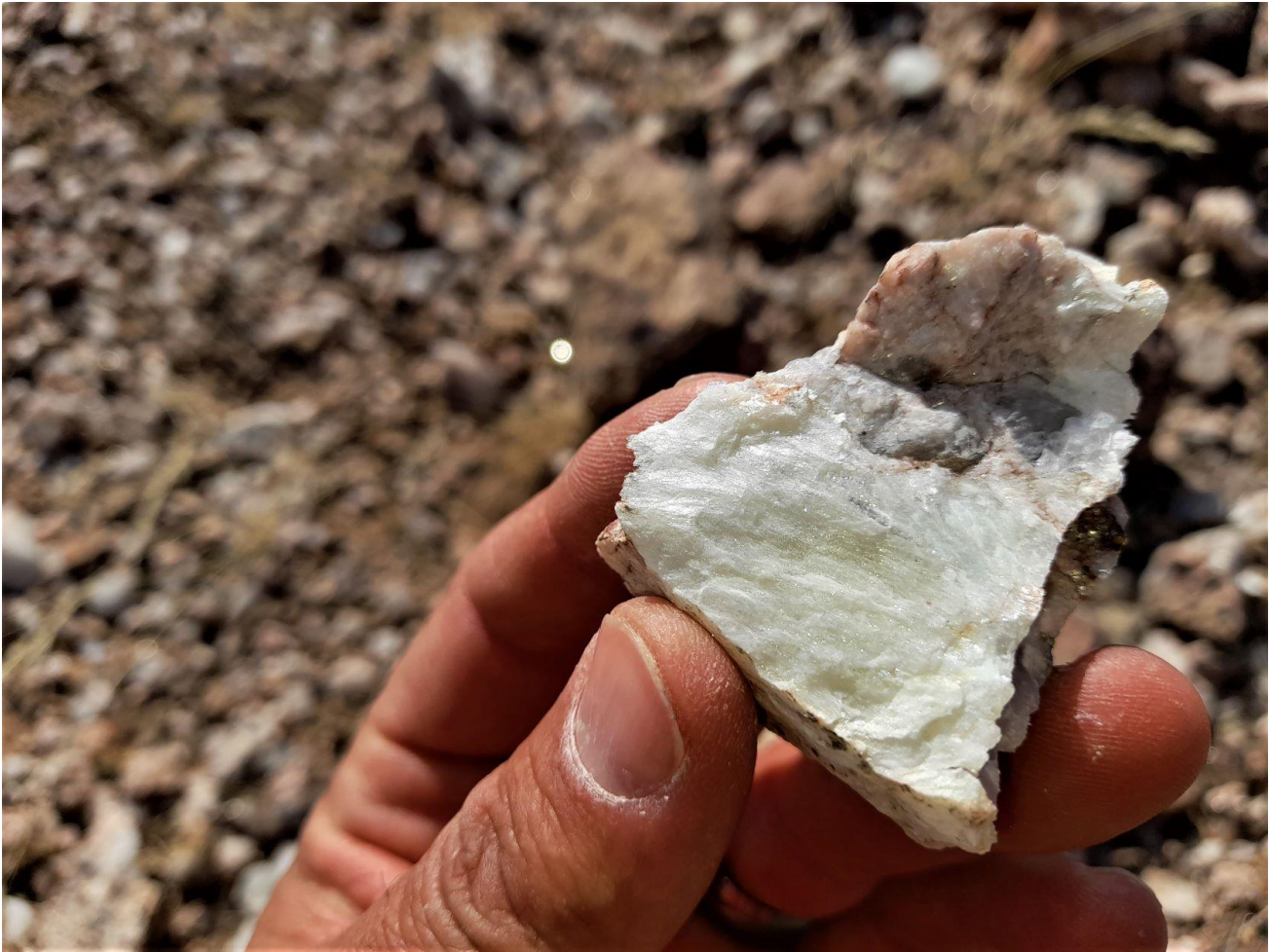
Figure 9: Sample containing unaltered spodumene collected from EPL 8535 during the October / November 2022 due diligence field sampling campaign - Note: Visual estimates should not be considered a proxy or substitute for laboratory analysis. Assay results are expected to be received in January 2023, subject to turnaround times at the laboratory. Sample Tag: U4674; Sample location – E: 472460 and N: 7639905
