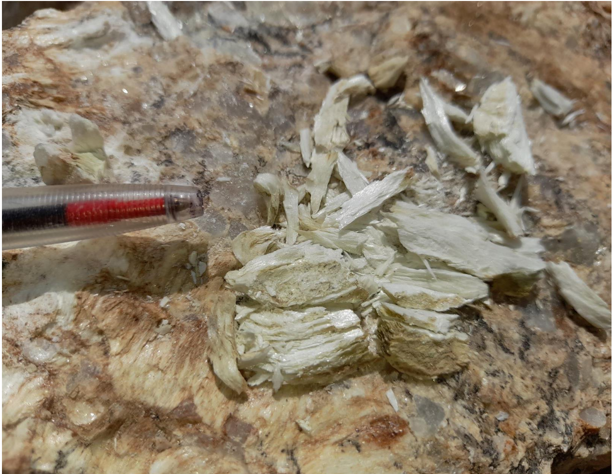
Figure 3: Example of fresh spodumene needles [close-up] identified at a pegmatite mine working located on EPL 8535 [Uis Lithium Project] - Note: Visual estimates should not be considered a proxy or substitute for laboratory analysis. Assay results are expected to be received in January 2023, subject to turnaround times at the laboratory. Sample Tag: U4797; Sample location - E: 480813 and N: 7635657
