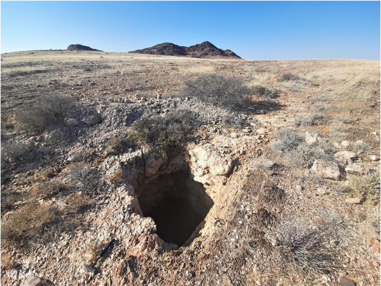
Figure 10: Deep pegmatite mine working identified at EPL 8535 which was visited during the October / November 2022 due diligence field sampling campaign
