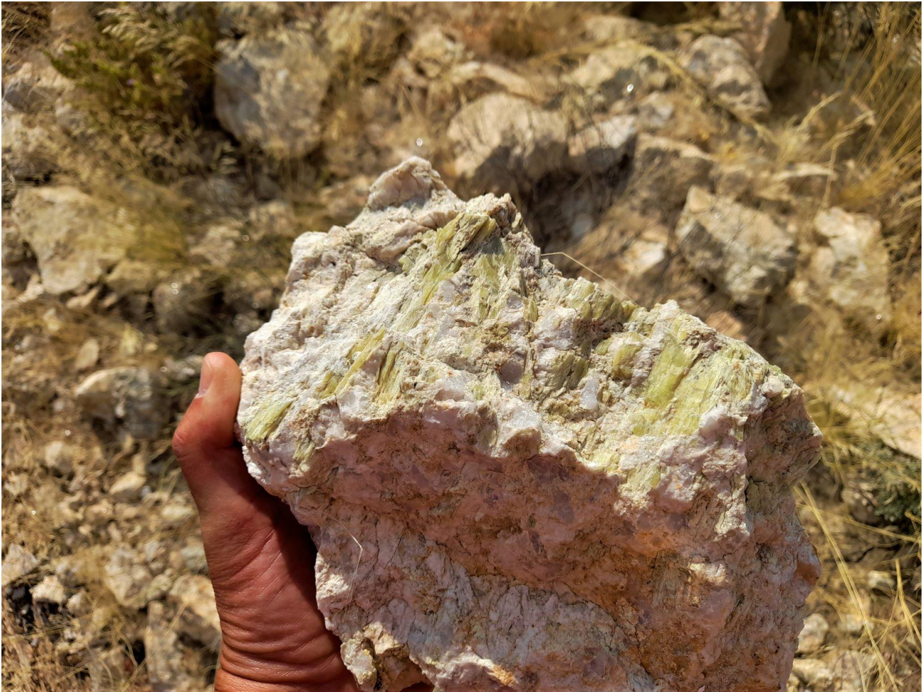
Figure 17: Example of altered spodumene mineralisation identified at EPL 8535 at a mine working visited during the October / November 2022 due diligence field sampling campaign
