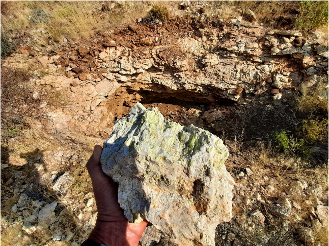
Figure 11: Altered spodumene, coloured in pale green, contained in a pegmatite outcrop collected during the October / November 2022 due diligence field sampling campaign at EPL 8535 - Note: Visual estimates should not be considered a proxy or substitute for laboratory analysis. Assay results are expected to be received in January 2023, subject to turnaround times at the laboratory. Sample Tag: U4685; Sample location – E: 472674 and N: 7639740
