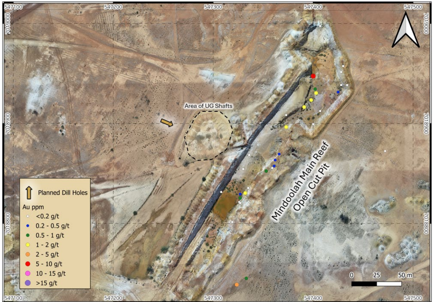
Figure 9. LiDAR imagery over Mindoolah Main Reef Open Cut Pit and surrounding Underground shafts with historic grab sample and Planned RC location in plan view (Appendix 1 – Table 2).
