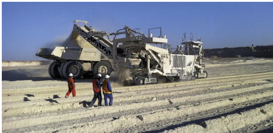
Fig 1 - Example Surface Miner – Limestone row cutting
