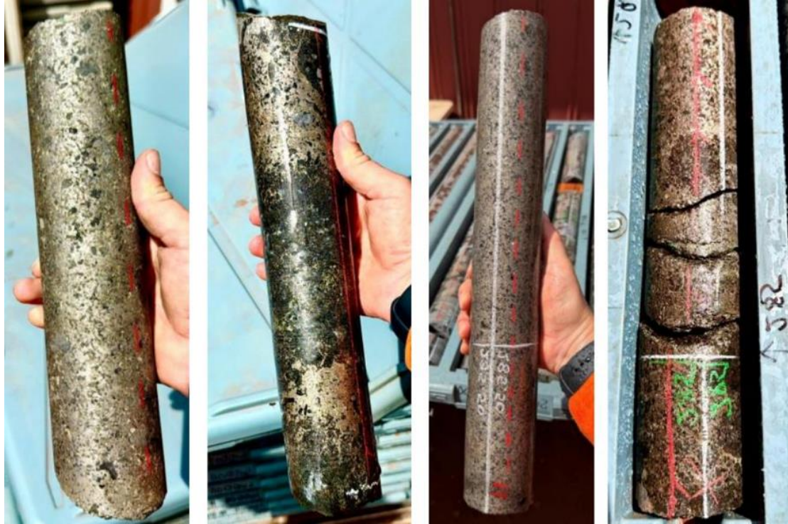
Figure 3. Massive to semi-massive sulfide intervals from SWDD011 at depths (from L-R) from 287.6-287.9m, 288.2-288.5m, 285.2-285.7m, 284.9-285.2m.
