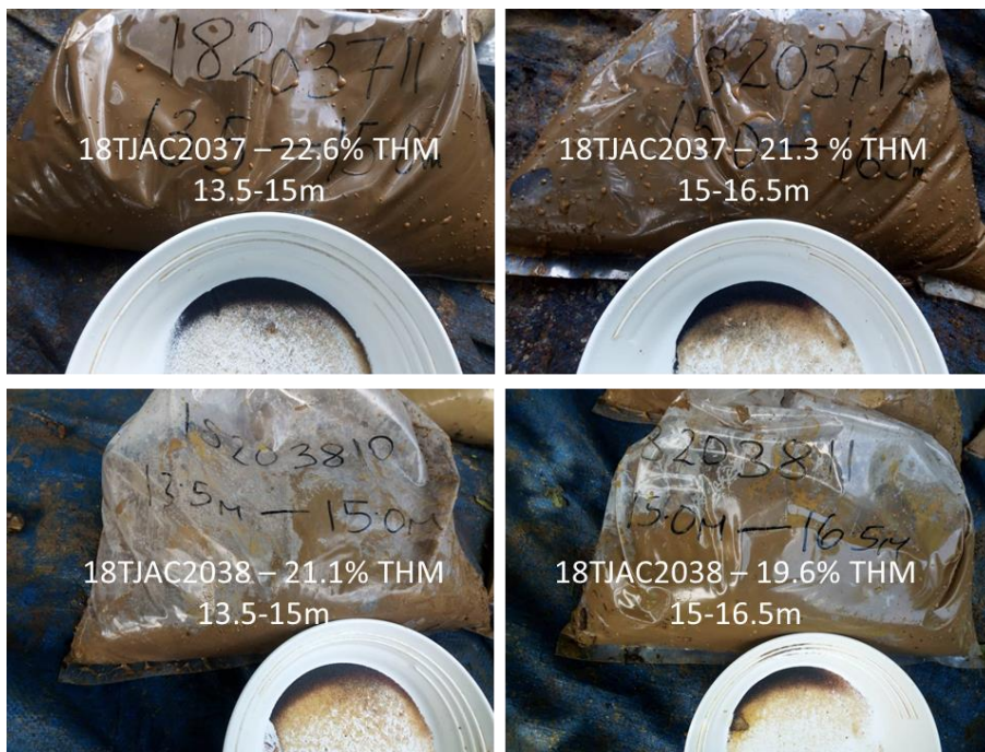
Figure 2 Panned samples from holes 18TJAC2037 and 18TJAC2038 within the high-grade trap site. The photos show the bagged samples as drilled and panned from the field with the laboratory derived THM analysis superimposed over the image. Refer to Figure 6 for a cross-section.
