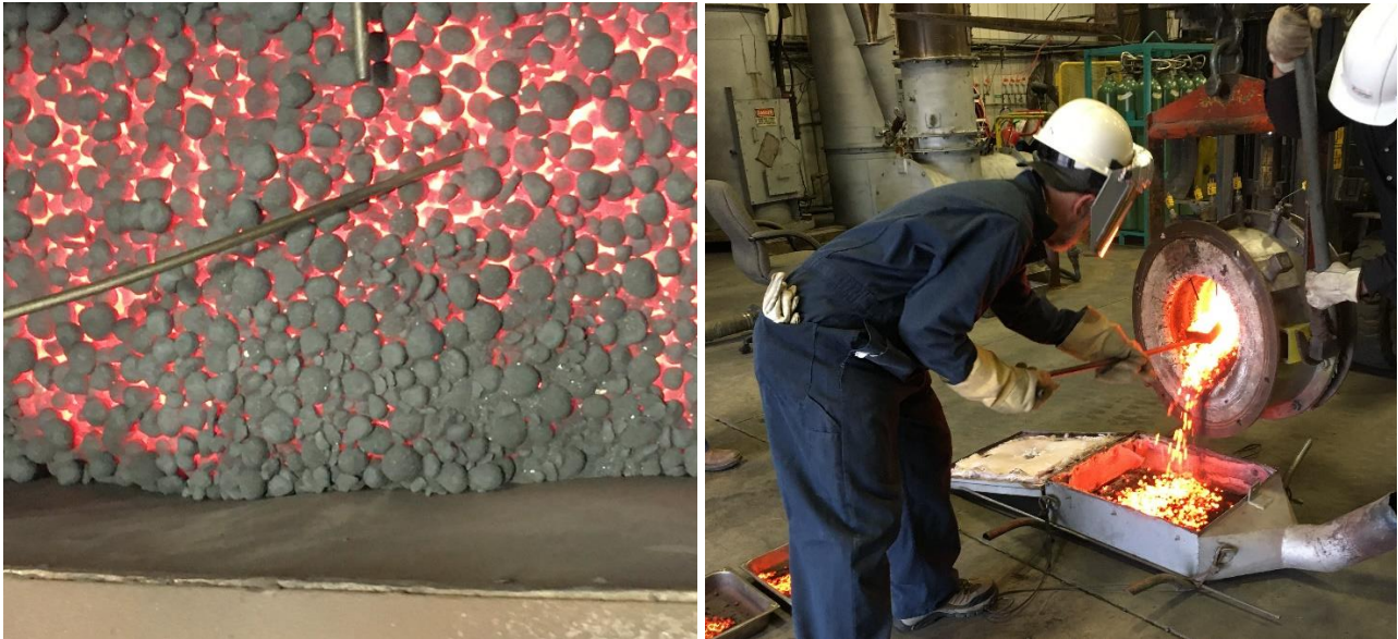
Figure 20 Roasting pellets of vanadium concentrate at Metso's pilot facility, Pennsylvania, USA
