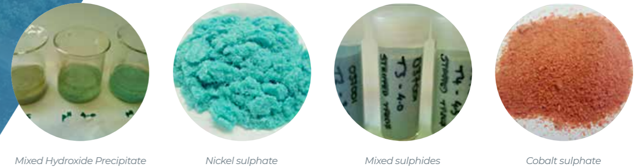
Figure 1 Nickel and Cobalt sulphate precipitated from Wingellina Ore during pilot test work completed in 2018
