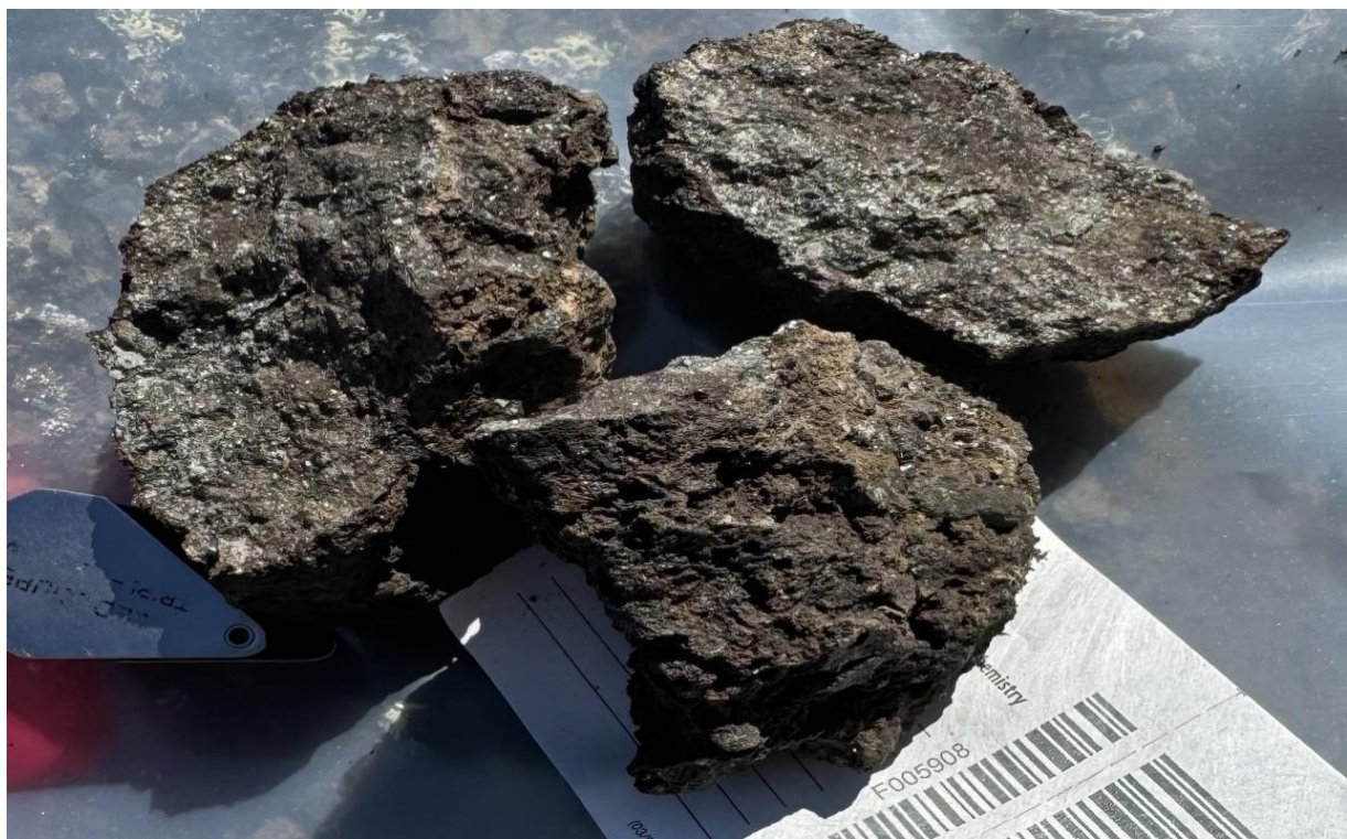
Figure 6 – Photograph of sample F005908, an intensely chlorite altered diorite with disseminated and vein hosted native silver which returned 9,070g/t Ag.
