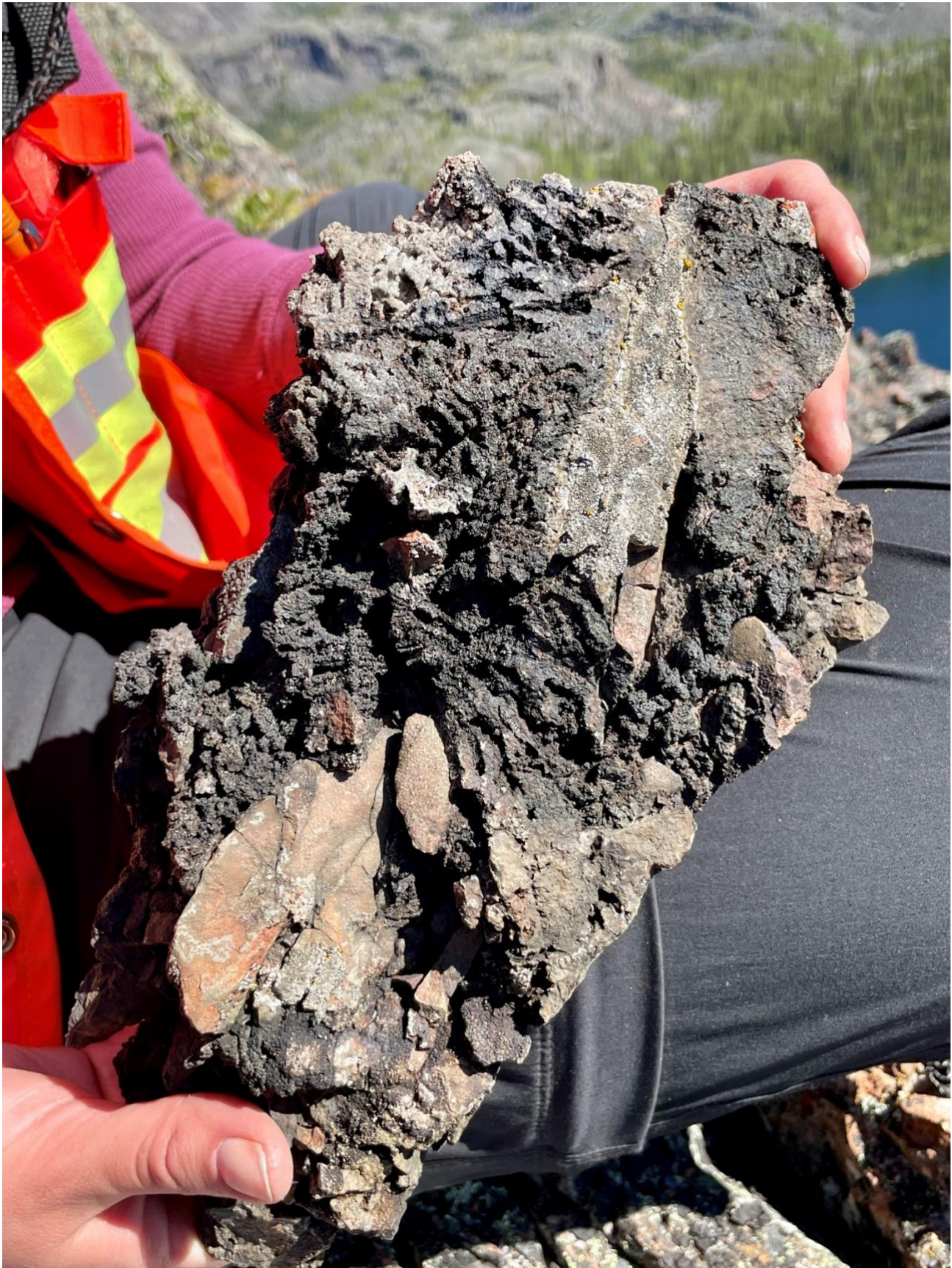
Figure 2 – Photograph of sample F005909 which returned 5.35% Ag. Tarnished native silver and calcite cement can be observed between the clasts of potassic altered diorite.
