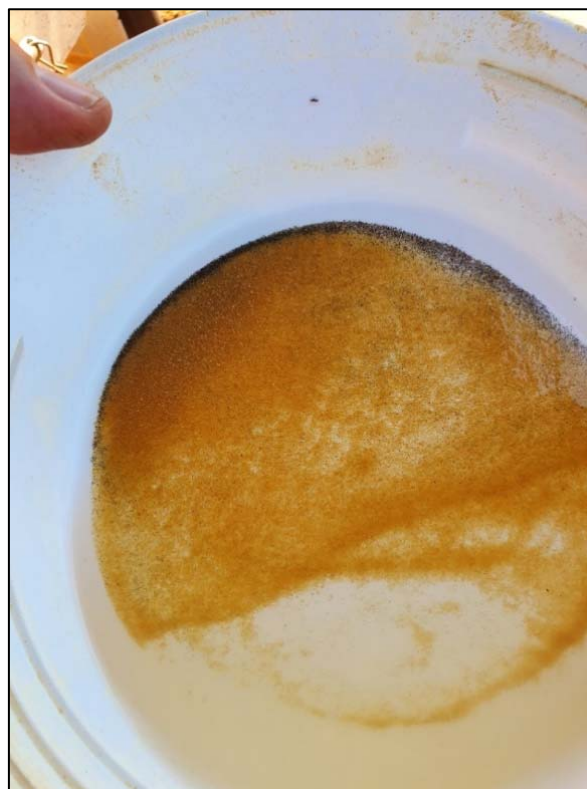
Figure 1 Typical panned sample taken from a higher-grade interval at Coburn Amy South drill program
