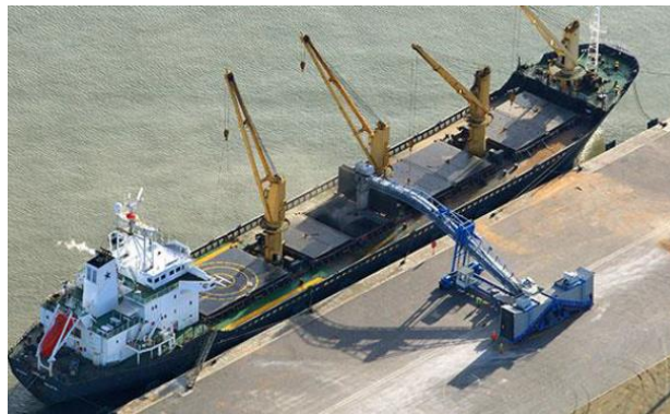
Image: Typical Mobile Dump Hopper and Shiploader
