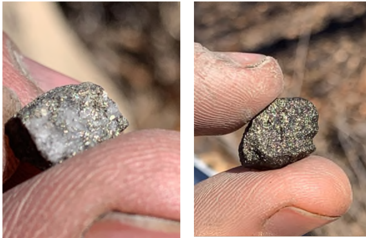
Figure 3: Selected RC drill chips from recent drilling program showing quartz+pyrite veining (L) and pyrite-rich black shale (R).
