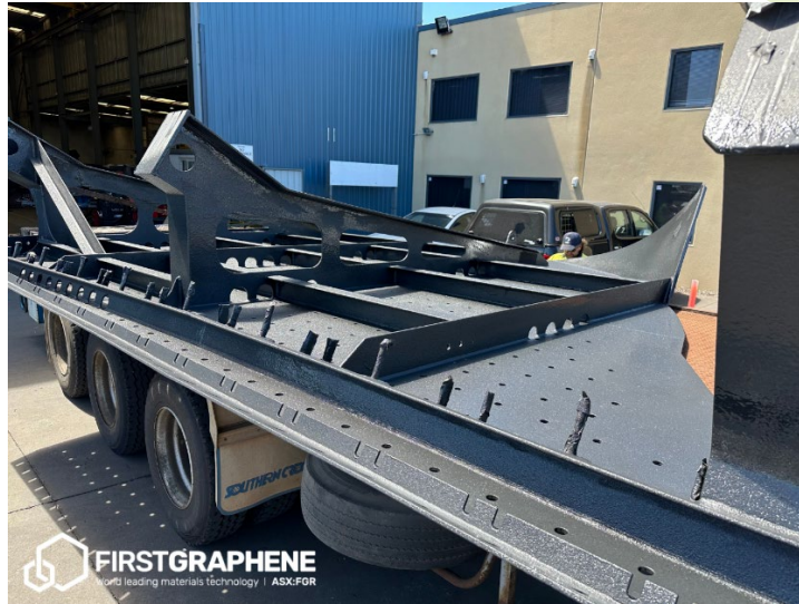
Figure 2: Chute panels coated with newGen's PureGRAPH® enhanced spray applied elastomer coating. Panels ready for dispatch to top tier mining companies operating in WA's North West.
