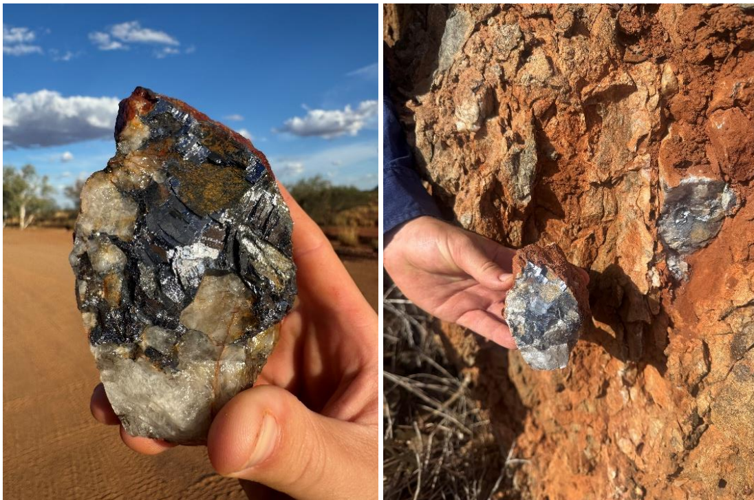
Figure 1: Galena (lead sulphide) in quartz vein from Thowagee Mine workings – to be assayed.
