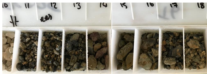
Figure 3 - RC Chips from BARRC025 (10-18m grading 0.9 g/t Au and 53 g/t Ag)
