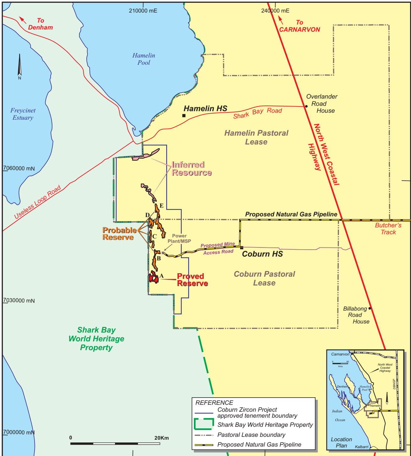
Figure 1 COBURN ZIRCON PROJECT - INFRASTRUCTURE
