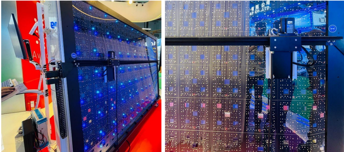
Image: Photographs of mockup large scale flash testing equipment.
