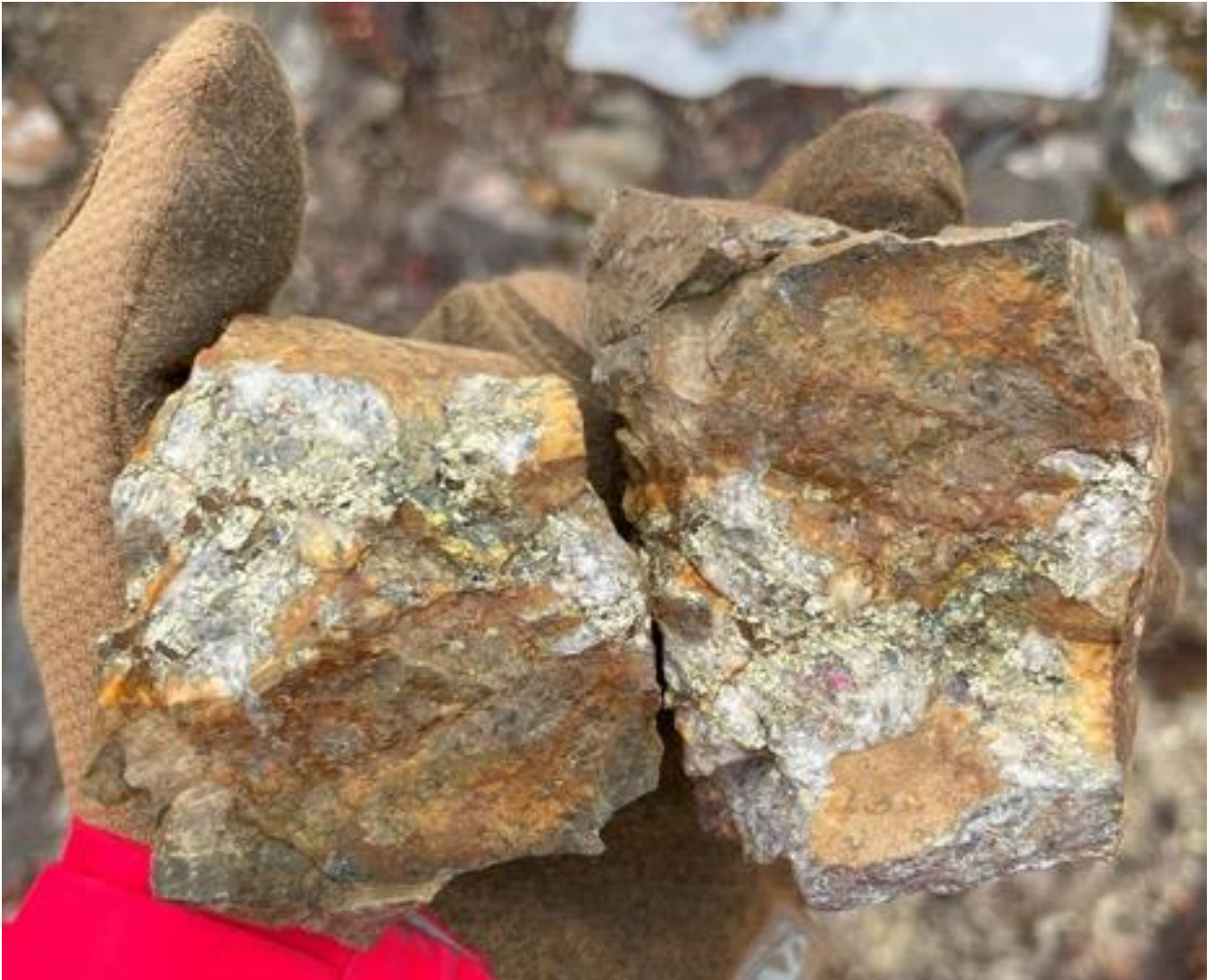
Figure 11 – Observed quartz-chalcopyrite vein with minor bornite from the Glacier epithermal trend which has been sampled over 200m strike length.
