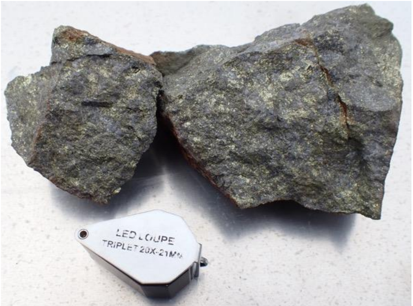
Figure 12 - Example of the Sparkplug Lake quartz-chalcopyrite veining which occurs within a 430 x 160m zone.
