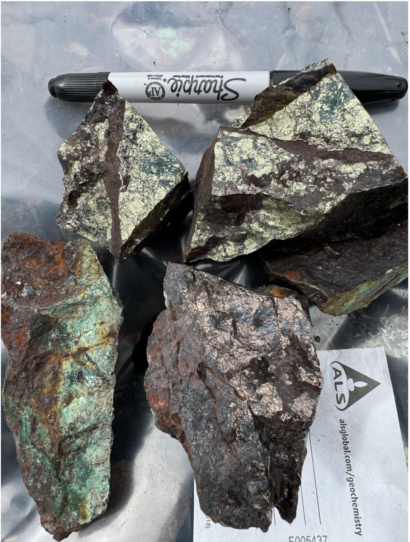
Figure 7 – Rock sample F005437 from a mineralised outcrop of massive chalcopyrite-bornite at the Glacier Target.
